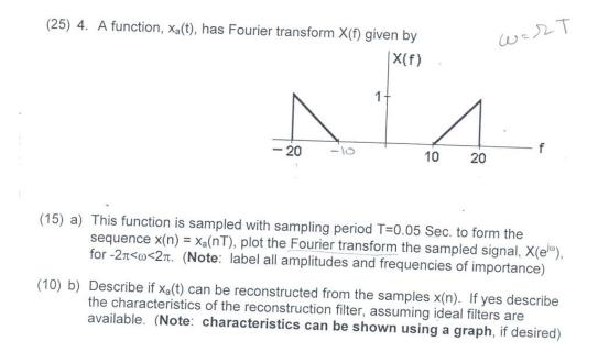
Maximum frequency in the signal can be seen to be 20Hz. Hence Nyquist frequency is twice this, which is 40Hz.
