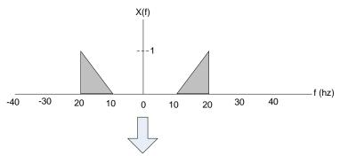
Duplicate at each multiple of sampling frequency, and scale
