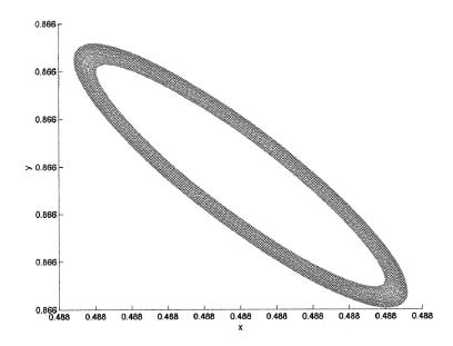
As it can be seen in the different plots, the motion of the spacecraft is the union of two circular motions, which result in a torus. Depending on how far we are from the equilibrium point, the torus has different shape. We can also realize that there are two periods present in the torus.
