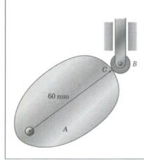
As cam A rotates, follower wheel B rolls without slipping on the face of the cam. Knowing that the normal components of the acceleration of the points of contact at C of the cam A and the wheel B are  $0.66 \text{ m/s}^2$  and  $6.8 \text{ m/s}^2$ , respectively, determine the diameter of the follower wheel.
