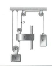
Block C starts from rest and moves down with a constant acceleration. Knowing that after block A has moved 1.5 ft its velocity is 0.6 ft/s, determine (a) the accelerations of A and C, (b) the velocity and the change in position of block B after 2 s.
