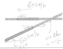
The velocities of commuter trains A and B are as shown. Knowing that the speed of each train is constant and that B reaches the crossing 10 min after A passed through the same crossing, determine (a) the relative velocity of B with respect to A, (b) the distance between the fronts of the engines 3 min after A passed through the crossing.
