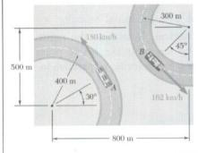
Racing cars A and B are traveling on circular portions of a race track. At the instant shown, the speed of A is decreasing at the rate of  $8 \text{ m/s}^2$ , and the speed of B is increasing at the rate of  $3 \text{ m/s}^2$ . For the positions shown, determine (a) the velocity of B relative to A, (b) the acceleration of B relative to A.
