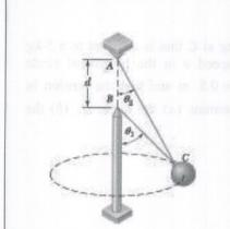
Two wires AC and BC are tied to a 15-lb sphere which revolves at a constant speed v in the horizontal circle shown. Knowing that  $\theta_1 = 50^\circ$  and  $\theta_2 = 25^\circ$  and that d = 4 ft, determine the range of values of v for which both wires are taut.
