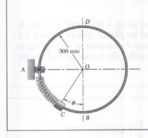
A thin circular rod is supported in a vertical plane by a bracket at A. Attached to the bracket and loosely wound around the rod is a spring of constant k = 40 N/m and undeformed length equal to the arc of circle AB. A 200-g collar C, not attached to the spring, can slide without friction along the rod. Knowing that the collar is released from rest when  $\theta = 30^{\circ}$ , determine (a) the maximum height above point B reached by the collar, (b) the maximum velocity of the collar.
