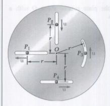
Four pins slide in four separate slots cut in a circular plate as shown. When the plate is at rest, each pin has a velocity directed as shown and of the same constant magnitude u. If each pin maintains the same velocity relative to the plate when the plate rotates about O with a constant counterclockwise angular velocity  $\omega$ , determine the acceleration of each pin.
