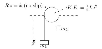
Since both masses will move with same speed  $\dot{x}$ , then the total kinetic energy of the system is
