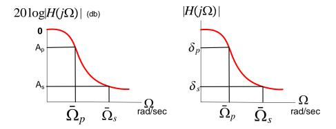
The specifications are given in db (the left diagram above) and not in magnitude (right diagram above). The specifications are given with reference to the transfer function magnitude. The phase is not taken into account in the specifications. Butterworth analog transfer function transfer function magnitude is given by
