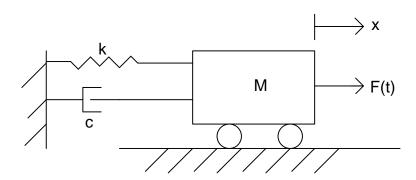
The first step is to obtain the equation of motion, which will be the second order ODE. Drawing the free body diagram and from Newton's second laws the equation of motion is found to be
